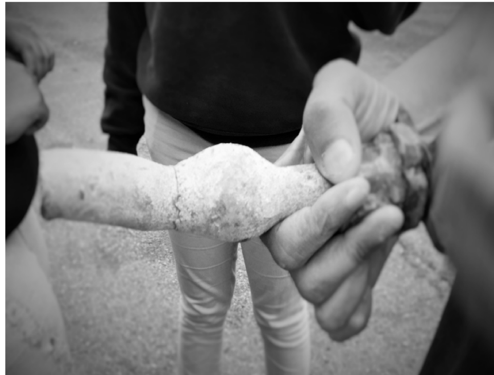
Part of a lead service line from a New Orleans home, Faubourg Tremé, 5/2/2016 -Credit: A. Katner
